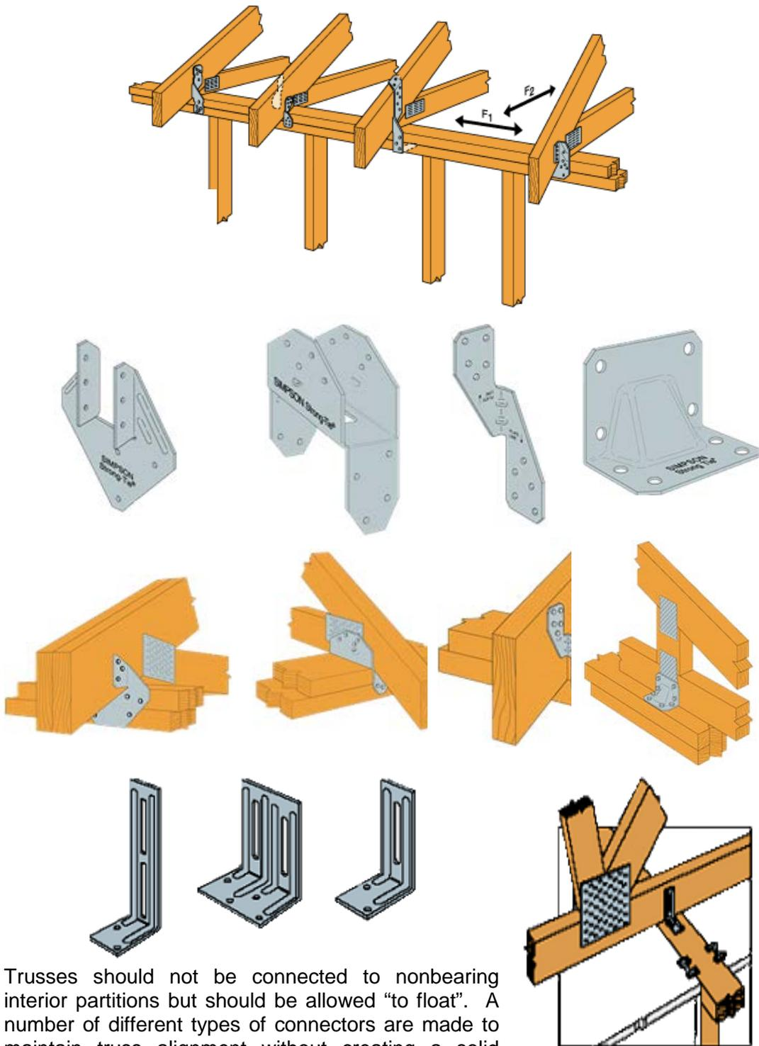
Trusses should not be connected to nonbearing interior partitions but should be allowed “to float”. A number of different types of connectors are made to maintain truss alignment without creating a solid connection. Nails installed in the slots should not be fully driven to allow the truss to move up and down.
